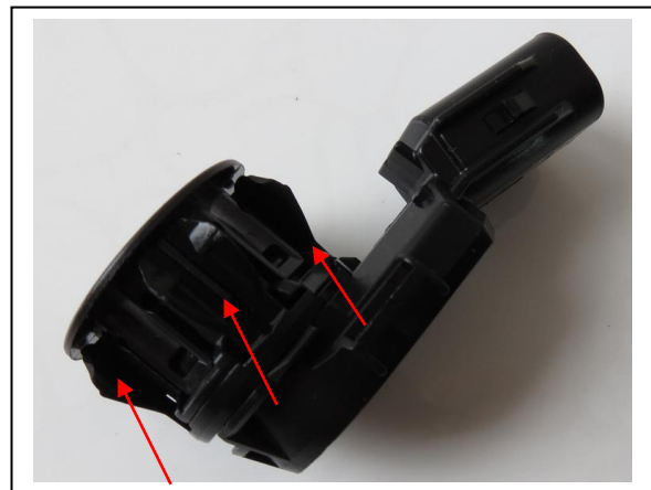
Figure 6: Remove centre parking sensor mounts
