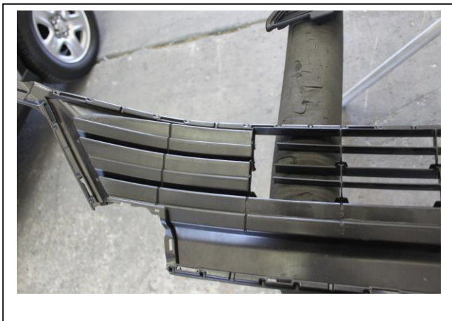
Figure 3: Trim grille for mounts to fit through
