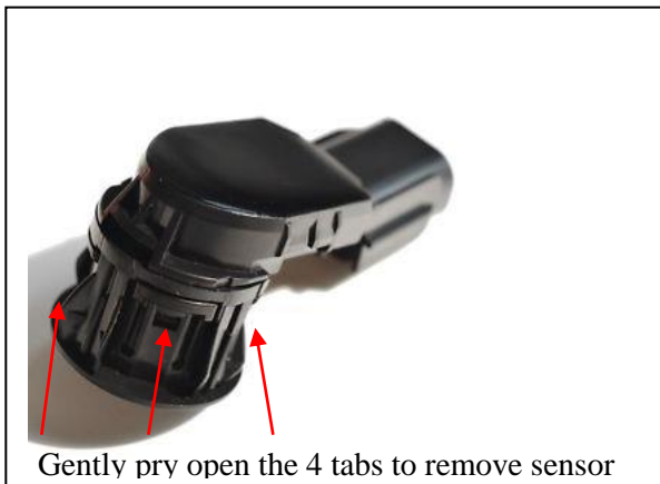
Figure 5: Remove centre parking sensors
