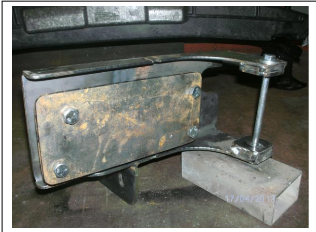
Figure 1: Rear of mount showing bolt direction. Bumper support removed for photo.
